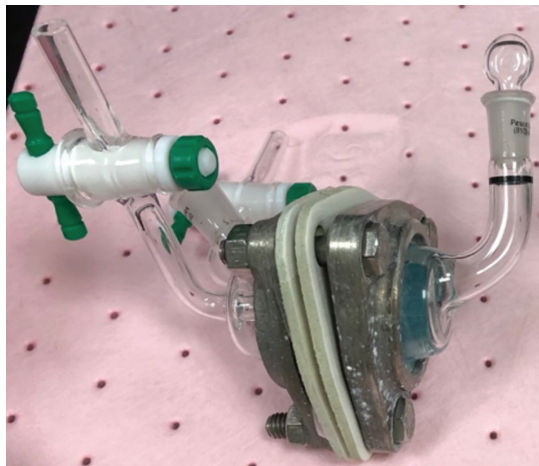
FIGURE 1B Exposure Test Chamber
